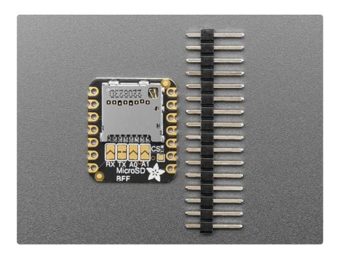
This PCB is designed to fit onto the back of any QT Py or Xiao board, it can be soldered into place or use pin and socket headers to make it removable. Onboard is a slim, high quality Molex push-pull micro SD card socket. Since the QT Py is already 3V, no level shifter or regulator is required. We're using SPI mode to interface, use the M OSI/MISO/SCK pins plus one other chip select pin. The default is TX but there are some solder jumpers you can use to select RX, A0 or A1.
