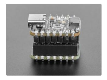
Connect the QT Py ESP32-S2 with pin headers into the microSD Card BFF with socket headers. They should be plugged in with the backs of the boards facing each other.
