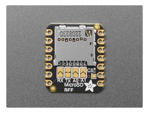
Adafruit QT Py boards are a great way to make very small microcontroller projects that pack a ton of power - and now there is a way for you to add a ton of storage, for reading and writing, with a micro SD card slot that can fit on the back of your miniature dev board. It uses the three SPI pins plus one chip select pin to access megs or gigs of data.
