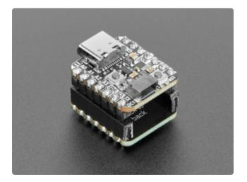
Connect the QT Py RP2040 with plug headers into the microSD Card BFF with socket headers. They should be plugged in with the backs of the boards facing each other.
