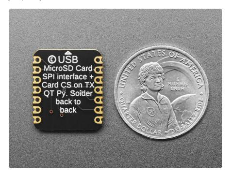
We include some header that you can solder to your QT Py. You can also pick up an <a href="Itsy Bitsy short female header kit to make it removable but compact">Itsy Bitsy short female header kit to make it removable but compact</a> (), you'll just need to trim down the headers to 7 pins long.
