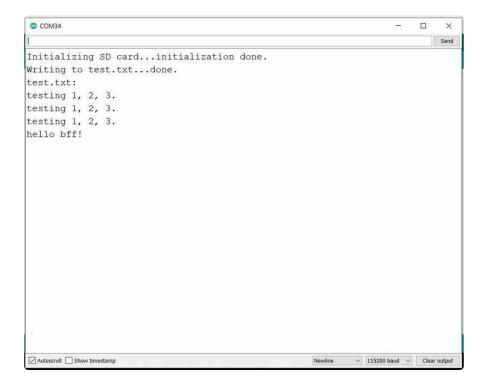
Upload the sketch to your board and open up the Serial Monitor (Tools -> Serial Monitor) at 115200 baud. A test text file will be created and written to on the SD card. Then, the text file will be read back with its contents printed to the Serial Monitor.
